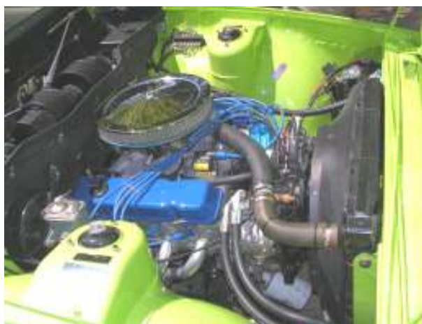
P76 engine (expanded to 5 litres) with Wilwood manifold, Rochester Quadrajet carburettor and Holden distributor (among other modifications)
